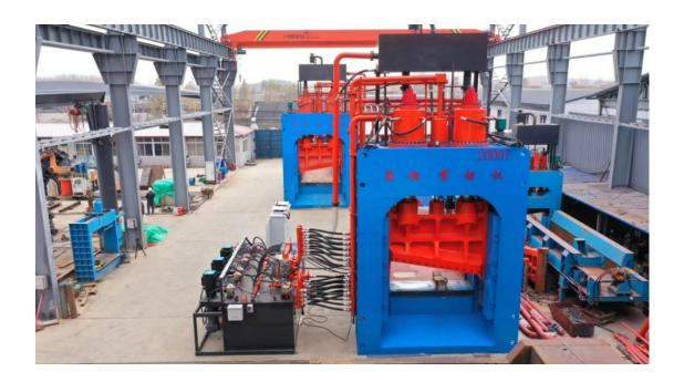
DL Industry Group Limited can produce the gantry guillotine shear with shear force 350T, 400T, 500T, 630T, 800T, 1000T, 1200T, 1400T, 1600T, 2000T, 2500T and customized one.
